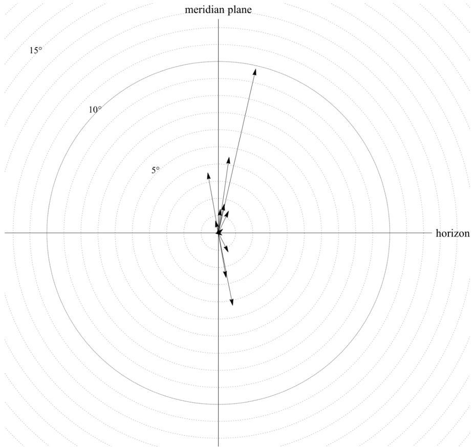
Fig. 4 Deviations of the cone axes towards the pole direction for well preserved conical sundials, based on the existing 3D models. The distances to the center indicates the deviation in the inclination, the directions of the arrows show their directions relative to the horizon and meridian line.
